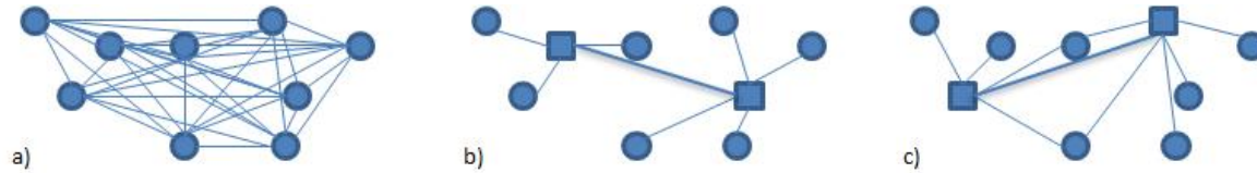
Figure 1.1: a) fully connected network b) single allocation hub and spoke design c) multiple allocation hub and spoke design.
