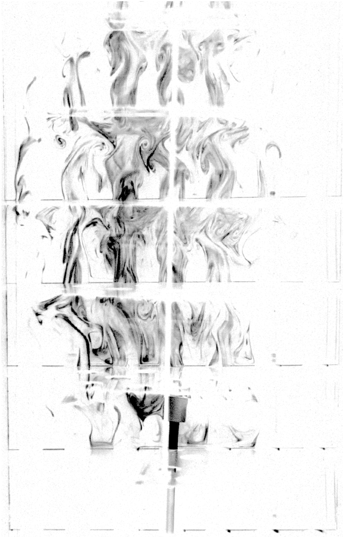
Figure 8.9: Net Flow Only in the 150 mm Multi-Orifice Apparatus, Re_n = 107 (Chaotic) 15 seconds after Dye Injection 1/30s at f2.8 6400ASA film
