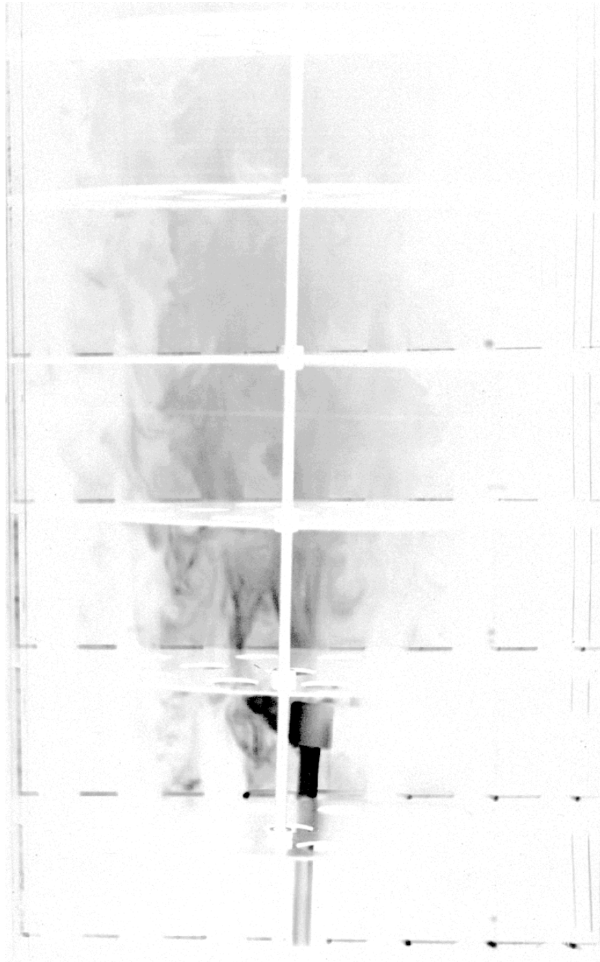
Figure 8.10: Net Flow Only in the 150 mm Multi-Orifice Apparatus, Re_n = 480 (Chaotic/Turbulent) 5 seconds after Dye Injection 1/30s at f2.8 6400ASA film
