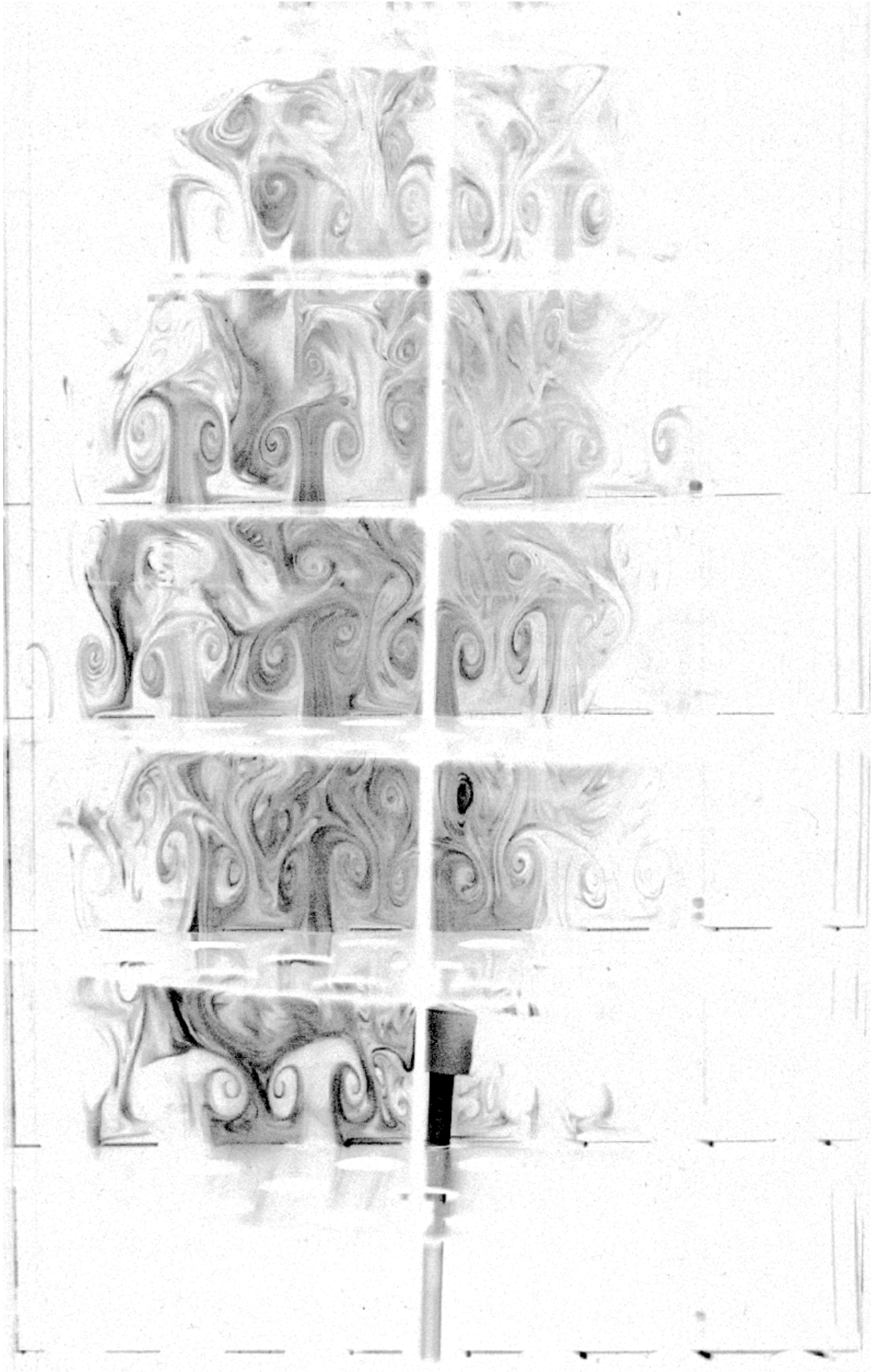
Figure 8.12: O.F.M. in the 150 mm Multi-Orifice Apparatus Re_n = 55 , Re_o = 75 and Str = 2 (0.5 Hz, 1 mm Oscillation) 1/30s at f2.8 6400ASA film
