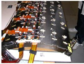
(a) Two harnesses mounted on the sector. The orange low mass tapes and black readout fibres are clearly visible.
