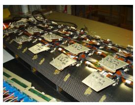
(b) The sector mounted with loopback cards, during harness testing.
