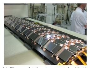
(c) The completed sector mounted with 48 barrel modules.
