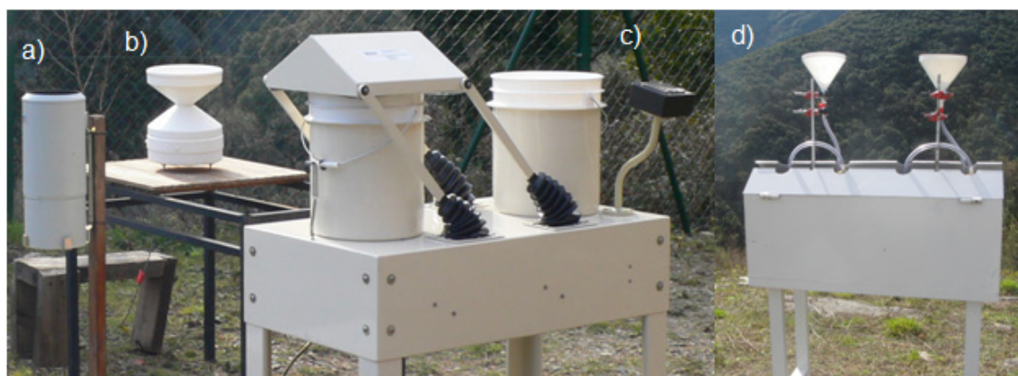
Figure 1. Atmospheric deposition sampling and precipitation measurement at LC: a) Hellman rain gauge; b) Campbell rain gauge connected to a data logger; c) Andersen wet/dry sampler (ESM Andersen instruments, G78-1001) and d) open bulk deposition collectors.
