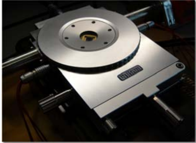
Figure 2.19: Linkam vacuum stage - This small chamber allows to heat and cool samples in a temperature range from -196^{\circ}\text{C} up to 350^{\circ}\text{C} and to perform vacuum testing at the same time.
