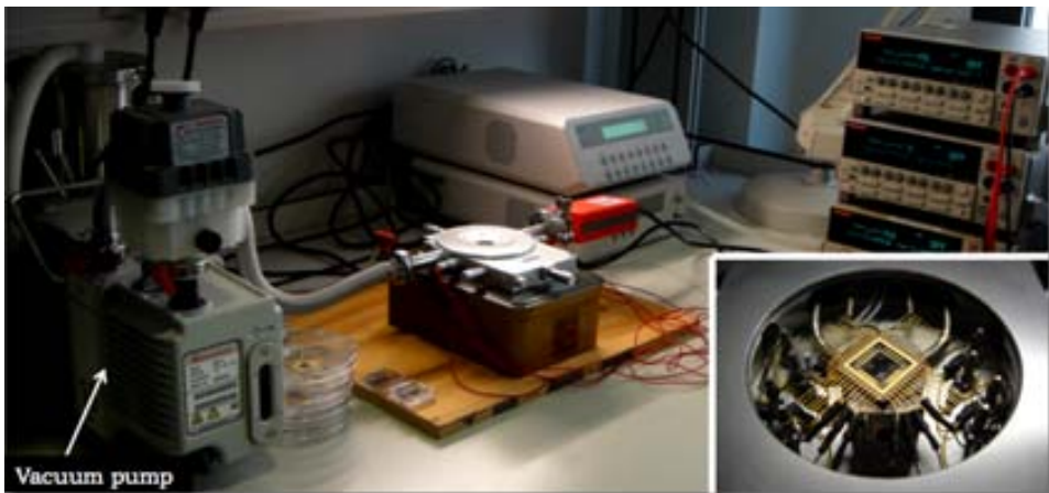
Figure 2.23: Set-up used for vacuum measurements - A rotatory vacuum pump with an active pirani gauge allowed to achieve vacuum levels of 10^{-3} mbar.
