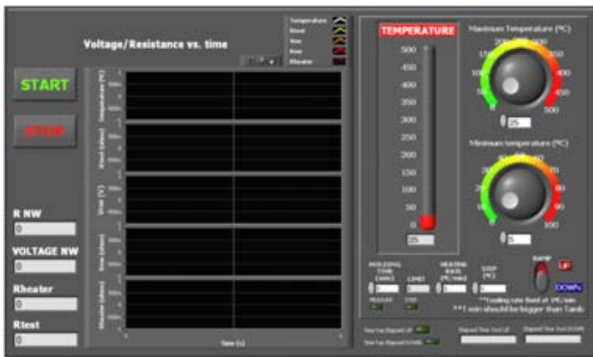
Figure 2.21: Screen shot of the program developed for I-V measurements for the harvesting mode - Interface of the program developed using LabVIEW software.
