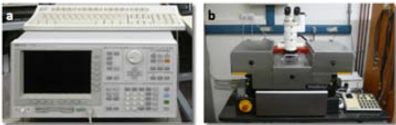
Figure 2.15: Electrical set-up used to performed four-probe measurements - (a) Semiconductor analyzer equipment used for resistance and voltage measurements. (b) System used to probe samples.
