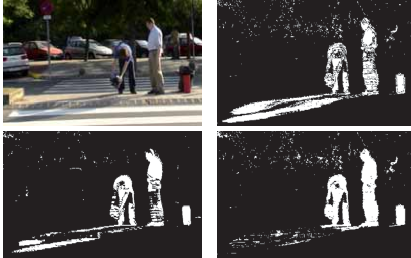
Figure 4.11: An original image from the Outdoor_Cam1 sequence, and foreground results after shadow removal using the Huerta et al. approach [25], the Zivkovic et al. approach [78] using a shadow detector [51], and our approach, respectively (read row-wise).
