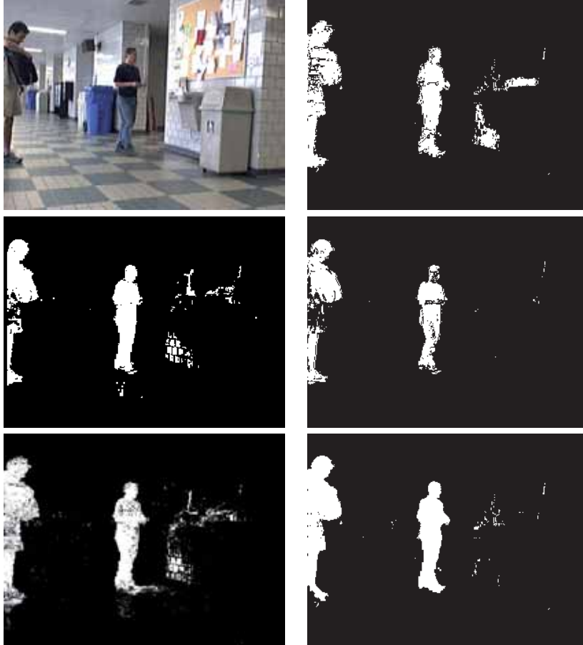
Figure 4.12: An original image from the HallwayI sequence, and foreground results after shadow removal using the Huerta et al. approach [25], the Kim et al. approach [33], the Zivkovic et al. approach [78] using a shadow detector [51], the Martel et al. approach [41], and our approach, respectively (read row-wise).
