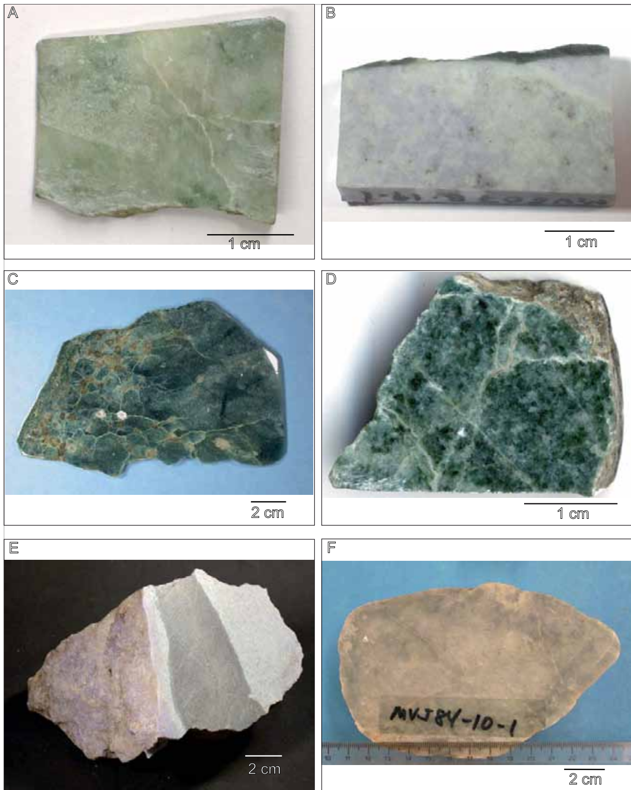
FIGURE 4 | Photographs of jadeitite hand-samples: A) Slab of whitish coarse-grained jadeitite: MVE04-44-2, Quebrada de los Pescaditos, 2.3cm wide; B) Slab of lavender jadeitite with pumpellyite at rim: MVE07B-19-1, near Saltán, 3cm across; C) Polished slice of jadeitite w/ large phengite grains and veins of blue-green omphacite: VMQ2-1, Quebrada Seca, Carrizal Grande, 15cm across; D) Polished jadeitite showing mottled dark green body cut by fractures and veins of cymrite and vesuvianite + cymrite: MVE02-17-5, La Ceiba, 3cm across; E) Sawn block of pumpellyite-jadeitite cut by a vein of brown chloritite: MVE03-76-4, Quebrada La Peña, La Ensenada, sawn surface is 20cm across; F) Slab of white-green medium-grained jadeitite with zones of translucent blue-greenish microcrystalline texture: MVJ84-10-1, Manzanal, ~14cm across.
