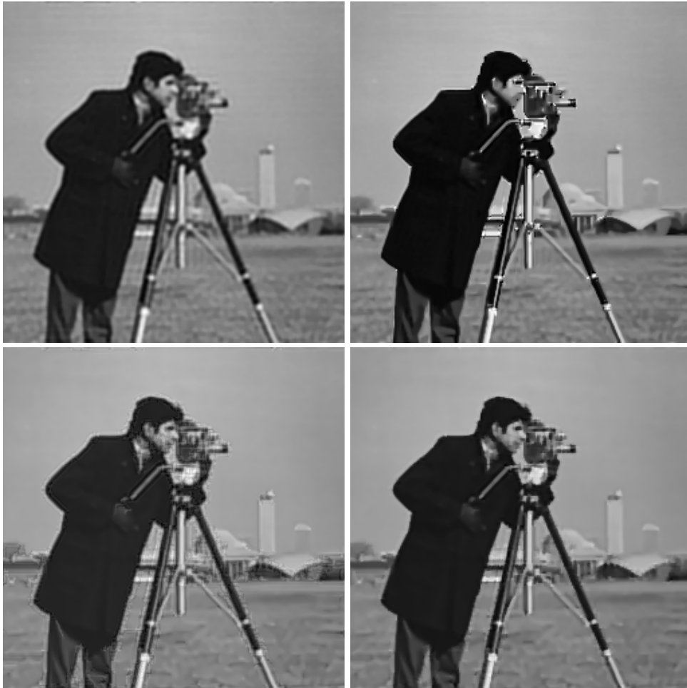
Figure 5: deconvolution results with different methods. Up left, FTVd [6] ISNR=2.4282, up right, NLTV [17] ISNR=4.3318, down left, NL-Re [18] ISNR=3.8777 and down right, the proposed algorithm ISNR=4.5260.
