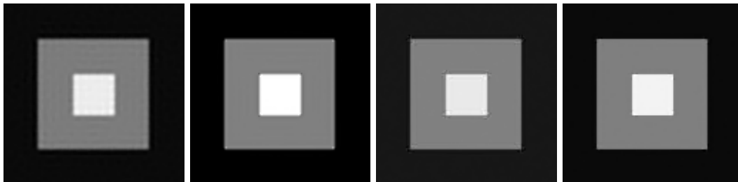
Figure 7: deconvolution results with different methods. From left to right: FTVd [6], NLTV [17], NL-Re [18] and the proposed algorithm.
