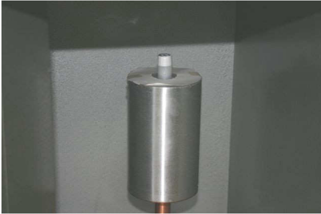
Figure 19: Interior of Ge well detector (gamma spectrometry) used for the measurement of ^{226}\text{Ra} and ^{228}\text{Ra} with a minivial at place.
