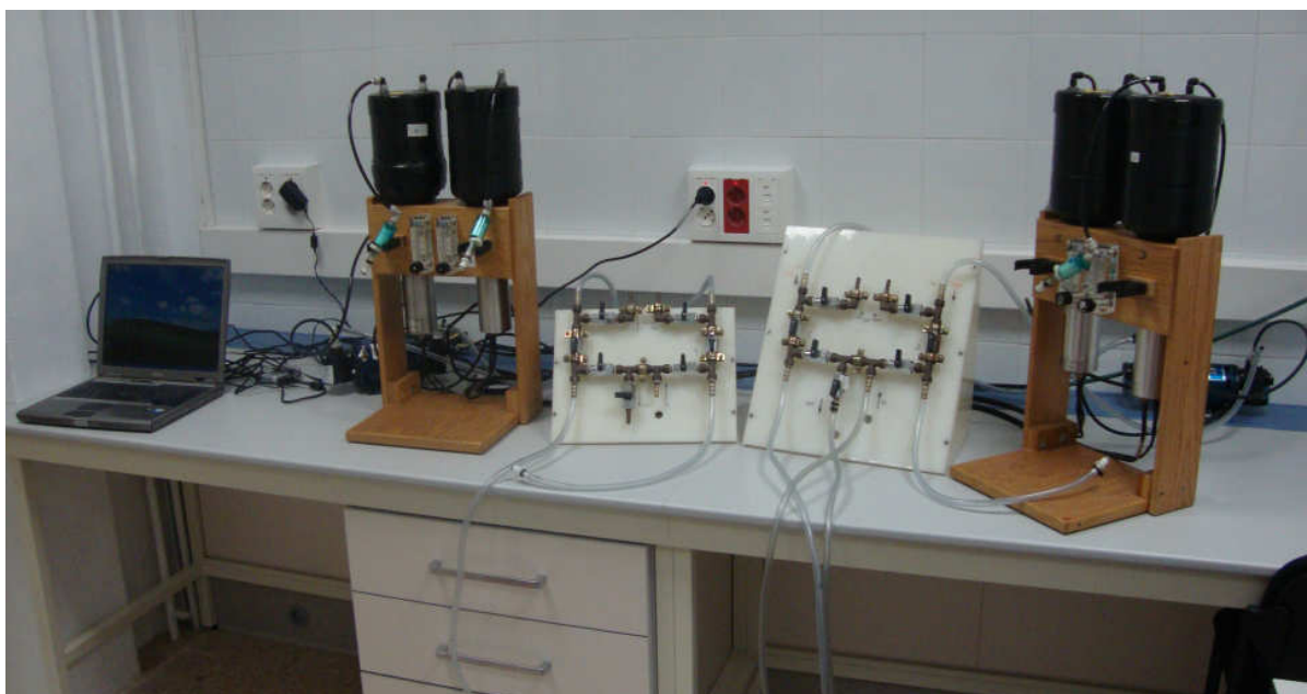
Figure. 18: RaDeCC equipment used for the measurement of ^{223}\text{Ra} and ^{224}\text{Ra} .
