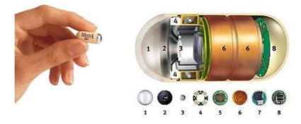
Figure 1.1: The M2AC camera (left) and the camera compontens (right) [15].
