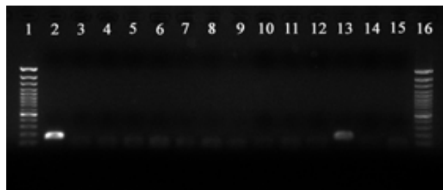
Figure 3.11 Lane 1: Fermentas GeneRuler™ 100 bp DNA Ladder, Lane 2: Positive control ( Nitrospira sp.), Lane 3: Negative control ( N.r winogradskyi ATCC 25391), Lane 4: Negative control (sterile MilliQ water), Lane 5 – 12: Reactor samples F_0 – F_7 , Lane 13: Positive control ( Nitrospira sp.), Lane 14: Negative control ( N. winogradskyi ATCC 25391), Lane 15: Negative control (sterile MilliQ water), Lane 16 : Fermentas GeneRuler™ 100 bp DNA Ladder.
