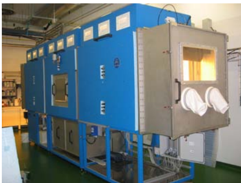
Figure 1.10 Unit of the Higher Plant Compartment (CIVb) installed in the MPP.
