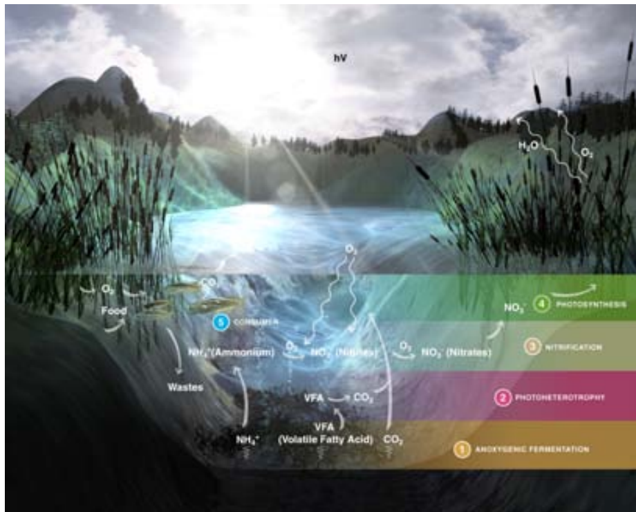
Figure 1.1 Scheme of the different biological functions in a lake ecosystem, providing the basis for the MELiSSA concept.
