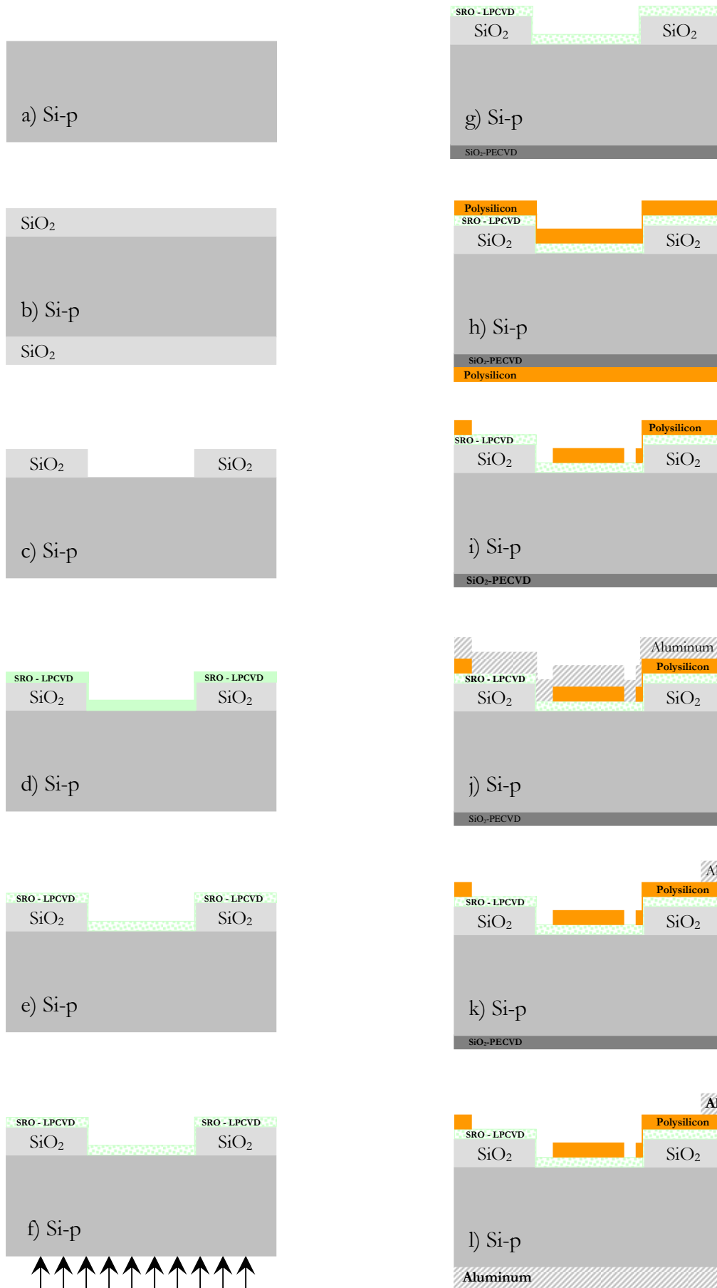
Figure 4.1. Fabrication steps of MOS-like structures.
