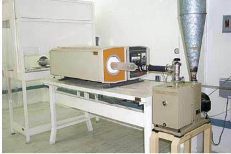
Figure 3.1. LPCVD system used for the deposition of SRO films from this work.
