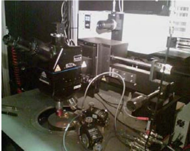
Figure 4.4. Schematic of the set-up used for pulsed EL measurements.
