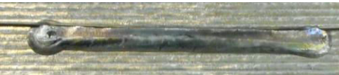
Step 2: Recharge line on the other side of the Ni coated FBG sensor The sensor is almost embedded in the tin alloy
