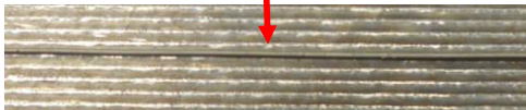
Step 1: Recharge line on one side of the Ni coated FBG sensor The sensor is partially embedded in the tin alloy
