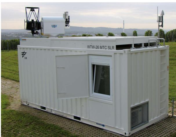
STAR-C: A platform raises a bi-static set-up of a wide field telescope and a laser transmitter above the roof of the container.
