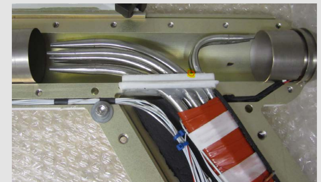
Figure 6. Photograph of HASI interior (position of air stream temperature sensor marked)
