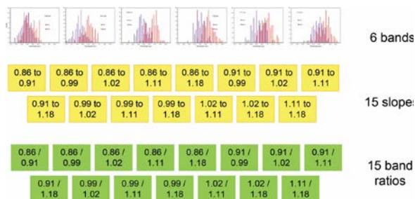
Figure 4. Parameterization of the information in the six emissivity bands collected by VEM into 36 values that contain predictive information, of which 21 are independent. The 36 values are then used in models to discriminate among rock types.
