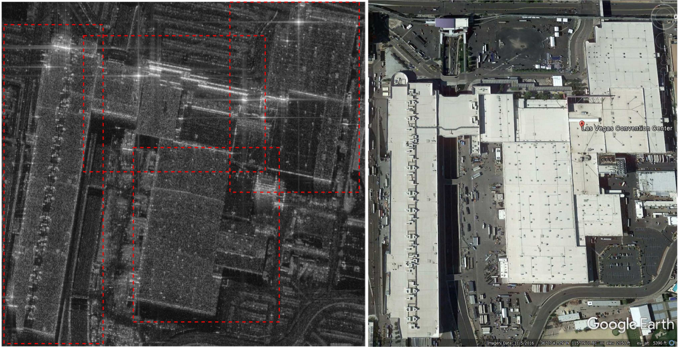
Fig. 13. (Left) TerraSAR-X test image of the Las Vegas Convention Center. Since the building structure is complex and its spatial area is large ( 800 \times 850 pixels), we separately process the four parts of the whole InSAR phase stack as cropped with the red dashed rectangles in the figure. (Right) Associated optical image from Google Earth.
