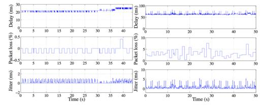
Figure 2. S-band link (left) and training setup (right) round delay measurements (DLR mission)
