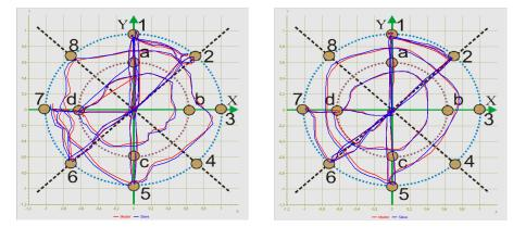
Figure 8. Trajectory of RJo's handle (Master) and Surikat (Slave) in the absence (left) and presence (right) of force feedback
