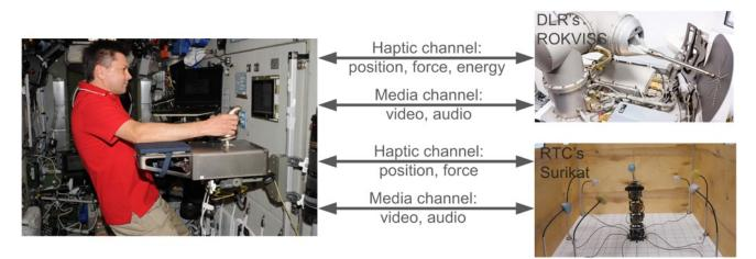
Figure 2. Telepresence data streams
