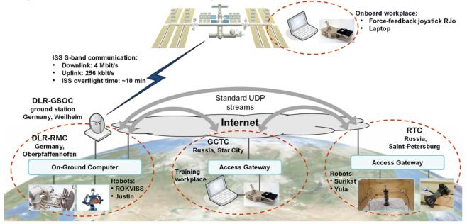
Figure 1. Space experiment setup
