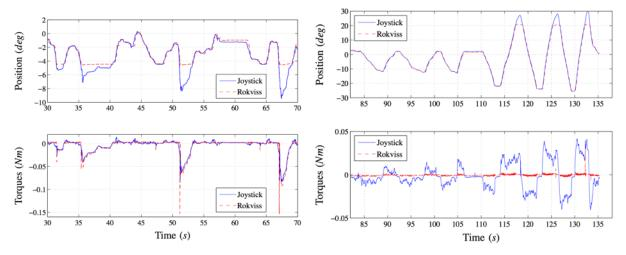
Figure 4. Position and force signals during one experimental session. Left: performance in hard contact situations. Right: performance in free space motion.
