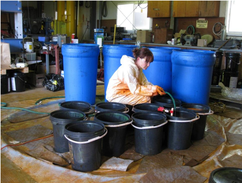
Figure 3-4: Transferring fluorescein concentrate to 5 gal. buckets for delivery to wells.
