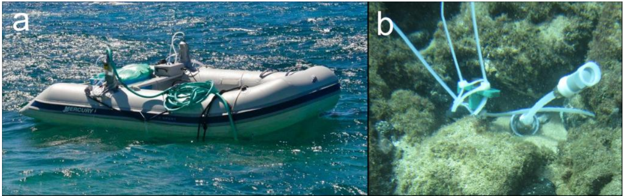
Figure 5-2: Photographs of the (a) time series zodiac and (b) piezometer with a hose connector installed in a submarine spring.
