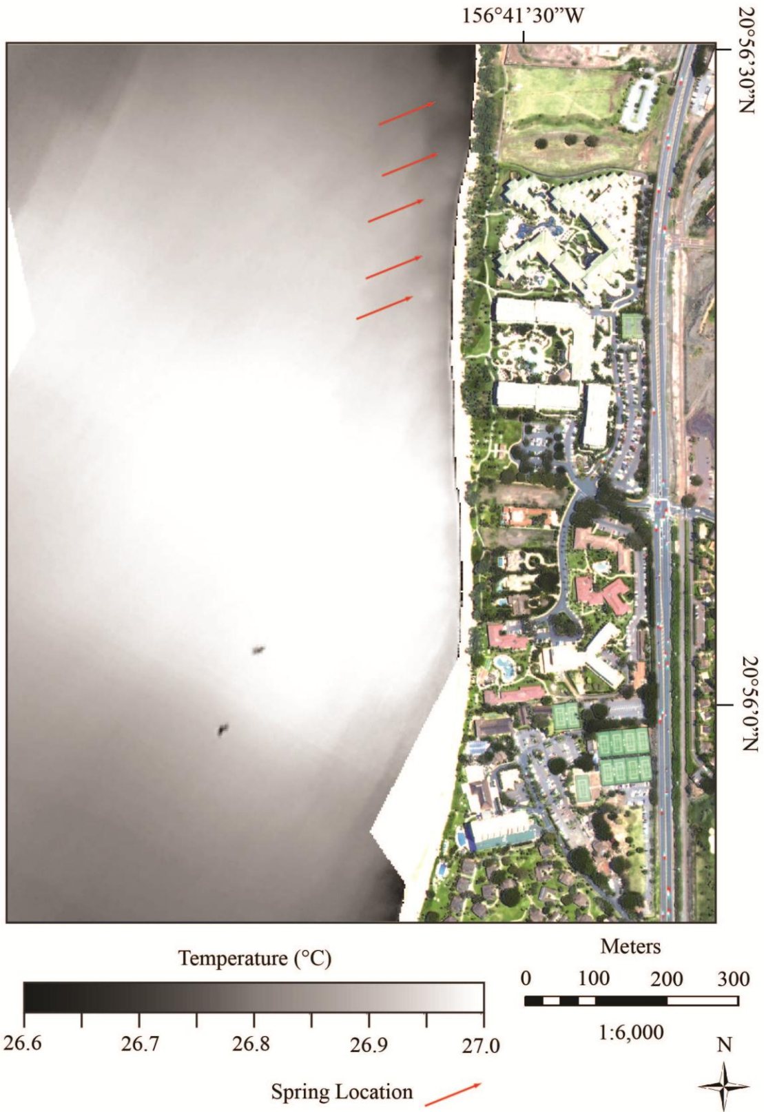
Figure 4-5: Submarine spring locations. Data are displayed on a gray-scale sea-surface temperature map.
