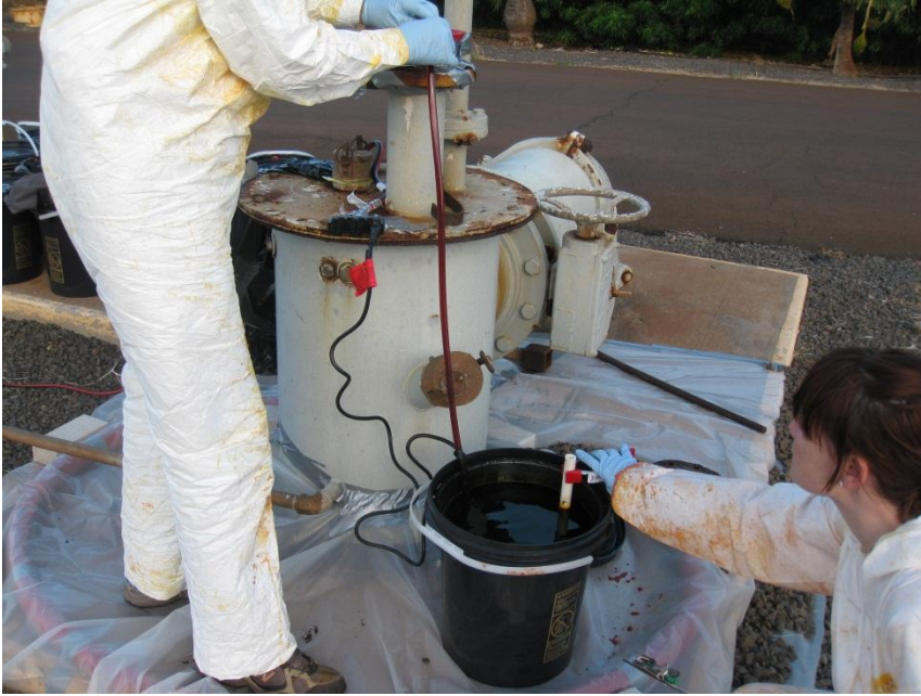
Figure 3-5: Transfer of dye concentrate into injection well 3.
