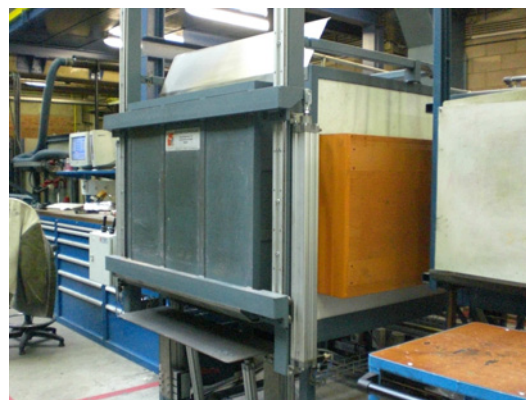
Figure 14 Oven to reheat the slabs
