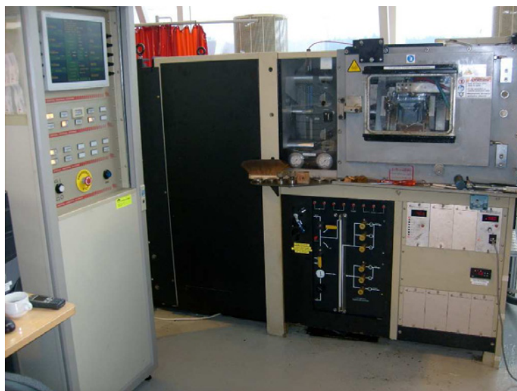
Figure 10 Gleeble 1500 D thermal cycle machine
