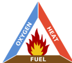
Figure 1.1: Fire triangle indicating the three elements that are required for a forest fire to burn. Taken from [4].
