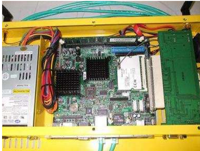
Figure 3.13: Wireless Node Architecture.
