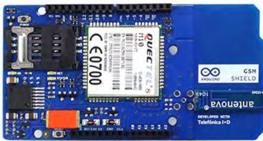
Figure 5 An Arduino GSM shield with a Quectel modem mounted
