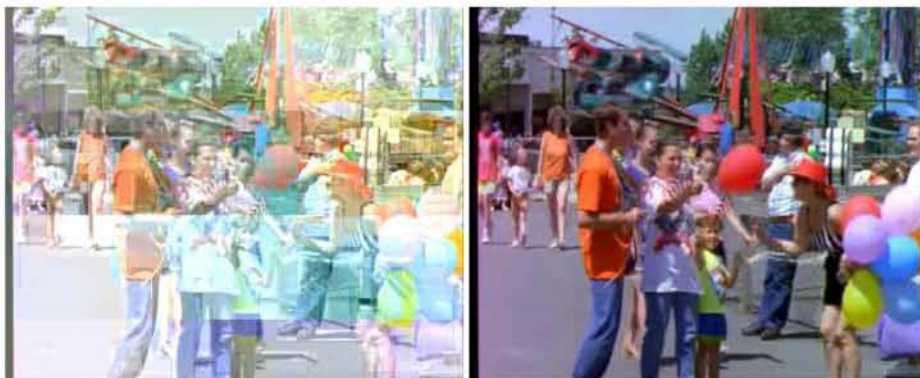
Figure A.2: Example output for fault injection in the AVS inverse transformation function. Left: top-left cell, right: bottom-right cell. All bits set to 0.
