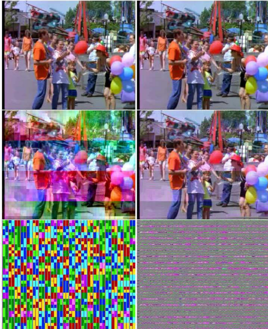
Figure A.3: Example outputs for fault injection in the AVS inverse transformation function. Left: top-left cell, right: bottom-right cell. Row 1, least significant bit (LSB) flipped. Row 2, 8th LSB flipped. Row 3, 16th LSB flipped.
