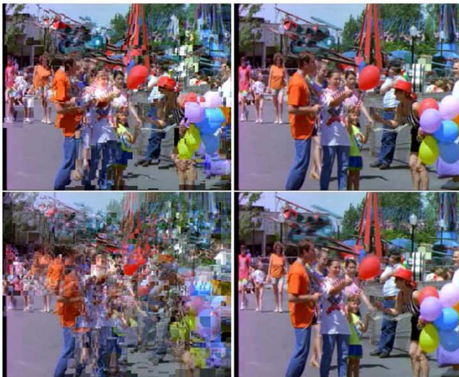
Figure A.5: Next 2 frames from the fault injection in the AVS motion vector values. Left faulted, right original
