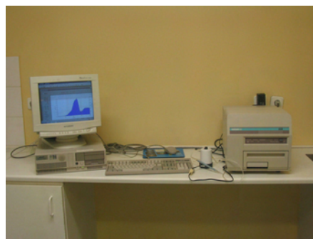
Figure 4.4: TLD reader and computer system
