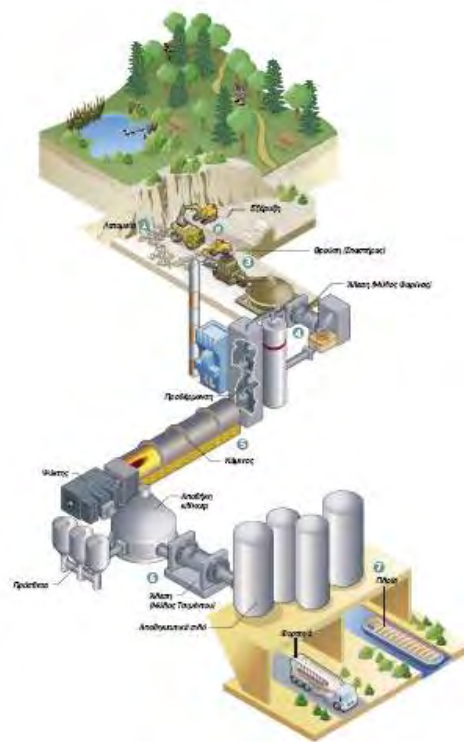
Figure 2.1: Basic flow sheet of cement production
