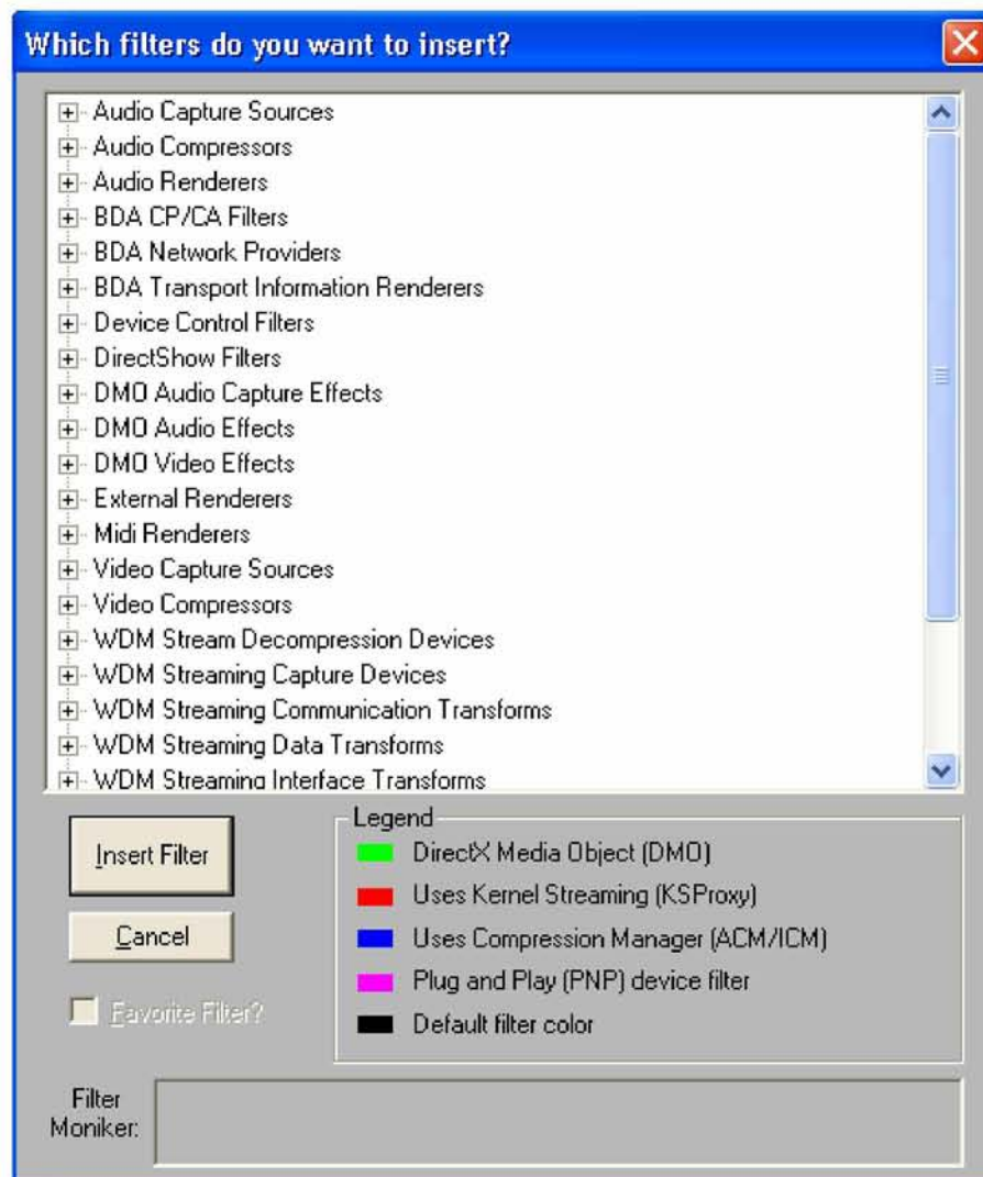
Figure 2-4. GraphEdit's Insert Filters dialog box enumerating all available DirectShow filters
