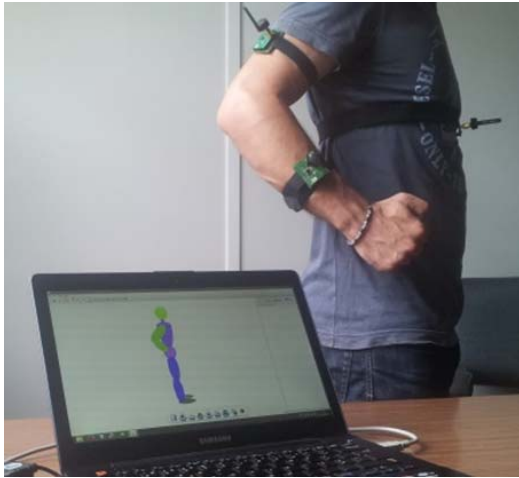
Fig. 6. Right arm movement replication, first position.
