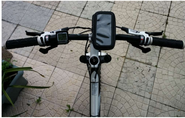
Fig. 6. Placement of the smartphone for the roughness test.
