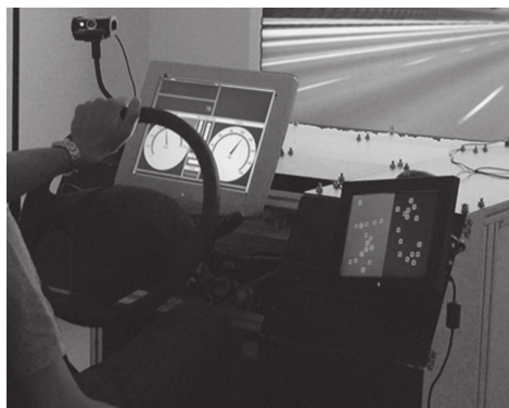
Figure 13.: Surrogate Visual Research Task on the right part of the driving simulator cockpit in Tango and Botta (2013).
