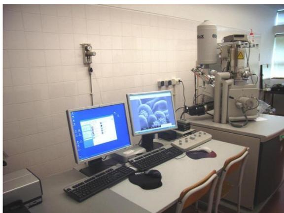
**Figura 4.1.** NanoSEM – FEI Nova 200 (FEG/SEM).
