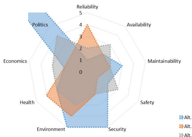
Figure 7. Spider plot as a possible result of multi-objective assessment of different maintenance alternatives against different performance aspects.
