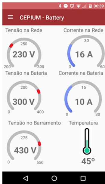
Fig. 3. App screen for presentation of the battery system sensor values.
