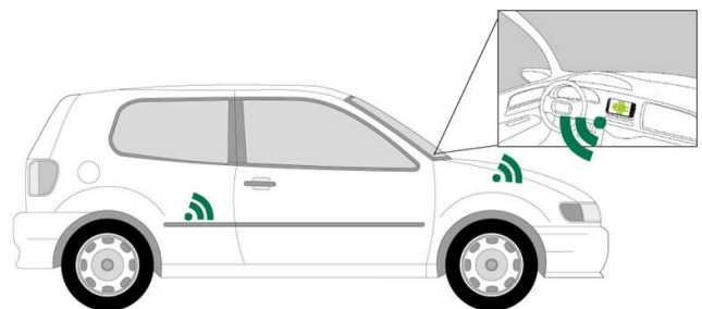
Fig. 2. Placement of the nodes of the BLE network inside of the car.
