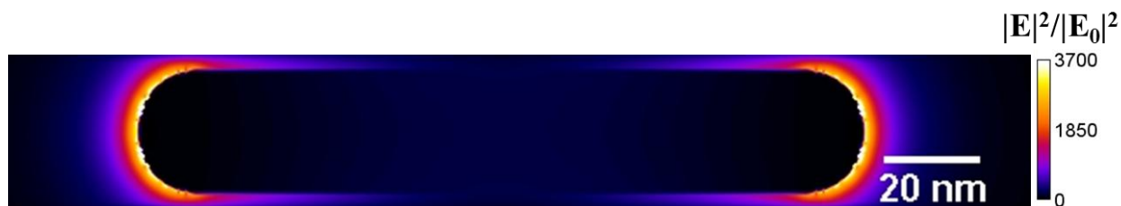
Figure 2.3. FDTD simulations of electric field enhancement at the surface of a gold nanorod. XY projection of calculated intensity. Simulations were performed for wavelength \lambda = 1064 nm, assuming that glass was the substrate. A gold nanorod with a 124-nm length and a 21-nm width is illuminated by light with linear polarization parallel to the longer axis of the gold nanorod. The colored scale bar represents the enhancement factor of the electric field relative to the incident field. The strongest enhancement is observed at the tips of the gold nanorod.
