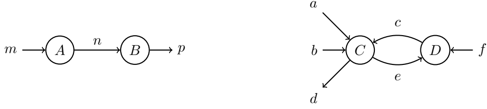
Figure 2.2: Graphical representation of a matrix-matrix product R_m^p = \sum_n B_n^p A_m^n (left) and a more complicated tensor product R_{abf}^d = \sum_{ce} C_{abc}^{de} D_{ef}^c (right).
