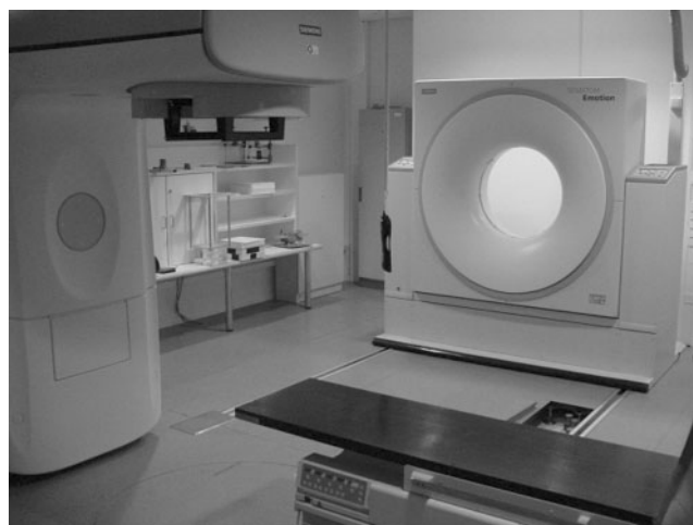
Figure 1. Treatment room with the Siemens Primatom at DKFZ Heidelberg. The linear accelerator and the CT scanner on rails share the same couch, which is rotated by 90° to switch between CT scanning and treatment position.
