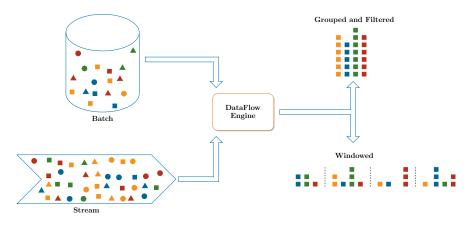
Figure 2.5: Batch and stream processing in the Google Dataflow model. Data may come as batch or from (potentially unaligned) data streams. It can be aggregated (for example filtered and grouped) or processed in windows over time.
