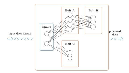
Figure 2.3: Apache Storm Topology with Spouts and Bolts as part of the stream processing. The spouts are sources of data, the bolts form different processing pipelines and transform the stream data, e.g. filter or aggregate it. Data is processed iteratively in single tuples, which allows low latency but limits throughput.
