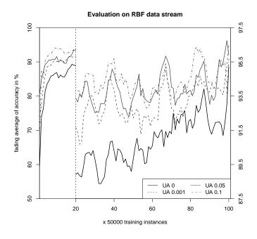
(a) HoeffdingAdaptiveTreePHT on RBF data stream with 5M instances.
