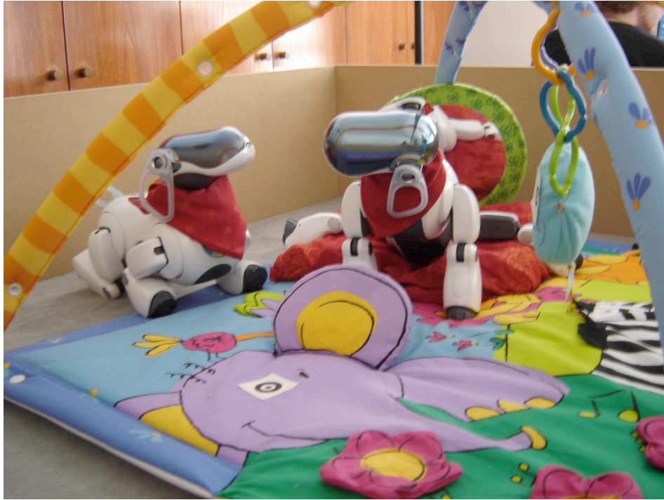
Figure 4 Curiosity-driven learning and self-organization of developmental structure in the Playground Experiment 22,28 . The robot in the center explores and learns to predict the effects of its actions, driven by an intrinsic motivation mechanism that drives it to focus on sensorimotor experiments that maximize learning progress/information gain. At the short time scale, this constitutes a model of curiosity-driven attention pushing the robot to prefer sensorimotor contingencies of intermediate complexity, compatible with recent experiments studying informational preferences in infants (Kidd et al., 2012). When running over an extended period of time, one observes the spontaneous self-organization of developmental phases of increasing complexity, without an initial program that specifies these phases. For example, the robot learns on its own to grasp an object in front of it, and later on focuses on exploring how to produce vocalizations that elicit reactions in another robot. Source: playground.png (Creative Commons)
