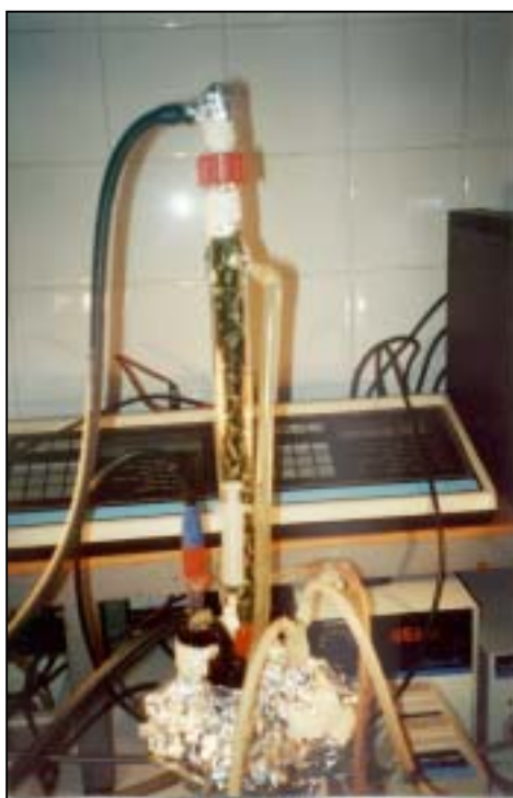
Figure 3.2. Image of the column with the biofilm developed from the lake sediment inoculum.
