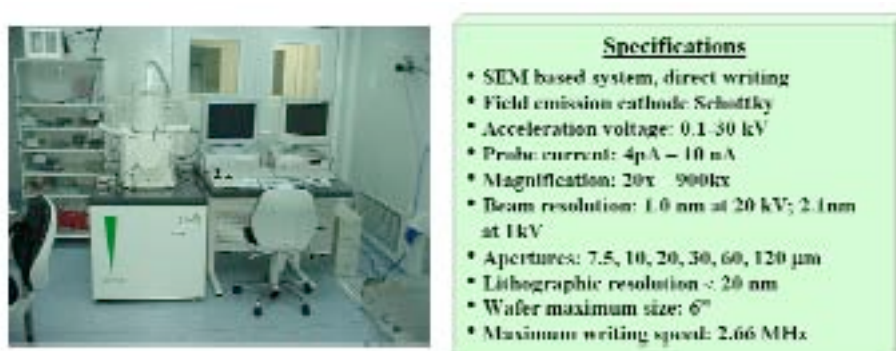
Figure 2.11 EBL system at the Nanofabrication Laboratory in the IMB-CNM.
