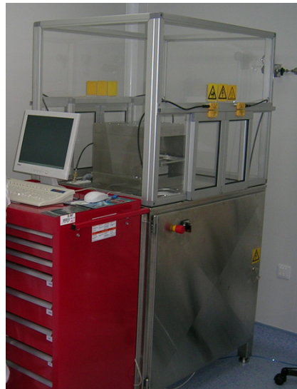
Figure 1.6. Nanoimprint Lithography (NIL) equipment from Obducat at the Nanofabrication Laboratory in the CNM.
