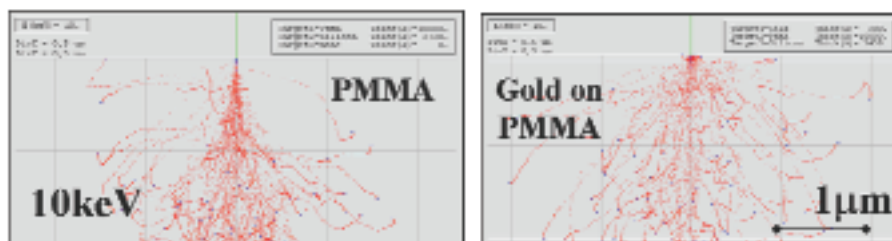
Figure 3.19 At 10 keV beam energy on 1µm thick PMMA, the inclusion of a 30 nm Au layer on the resist to avoid charging causes higher beam spread. Thinner metal layer and higher beam energies will improve the resolution.
