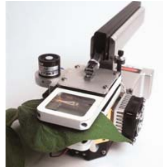
Figure 6.2 LI-6400 used for photosynthetic response to light at leaf scale.
