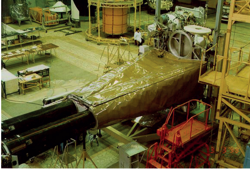
Figure 10. Covered part of the SODART optical block with two telescopes.
