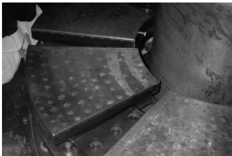
Fig. 3. Tilting-pads thrust bearing [8].
