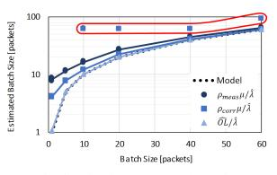
Fig. 6: Estimating the average batch size.
