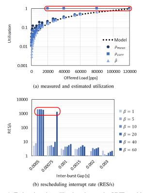
Fig. 4: Estimating the utilization due to the VNF workload.
