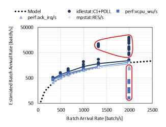
Fig. 5: Estimating the batch arrival rate using various PMCs.
