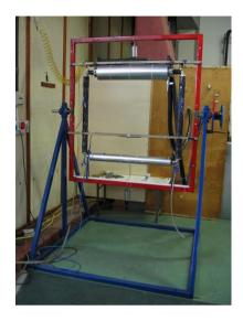
Figure 1. Experimental natural circulation loop [9]
