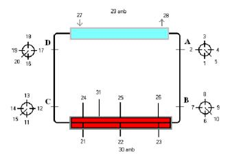
Figure 2. Thermocouples siting
