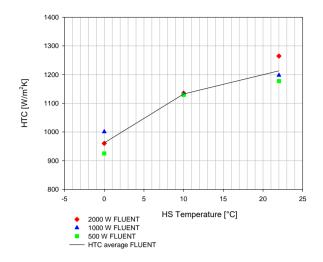
Figure 6. HTC vs. heat power and heat sink temperature (calculated by ANSYS FLUENT 3D simulations)
