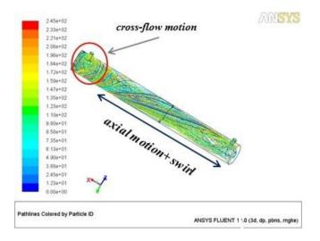
Figure 5. Pathlines water-glycol mixture inside cooler
