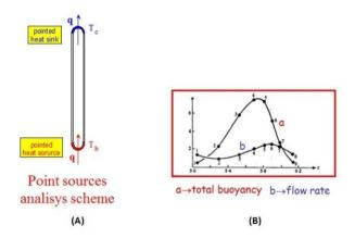
Figure 12. Welander's theory: (A) calculation scheme and (B) results graphic representation [5][16]
