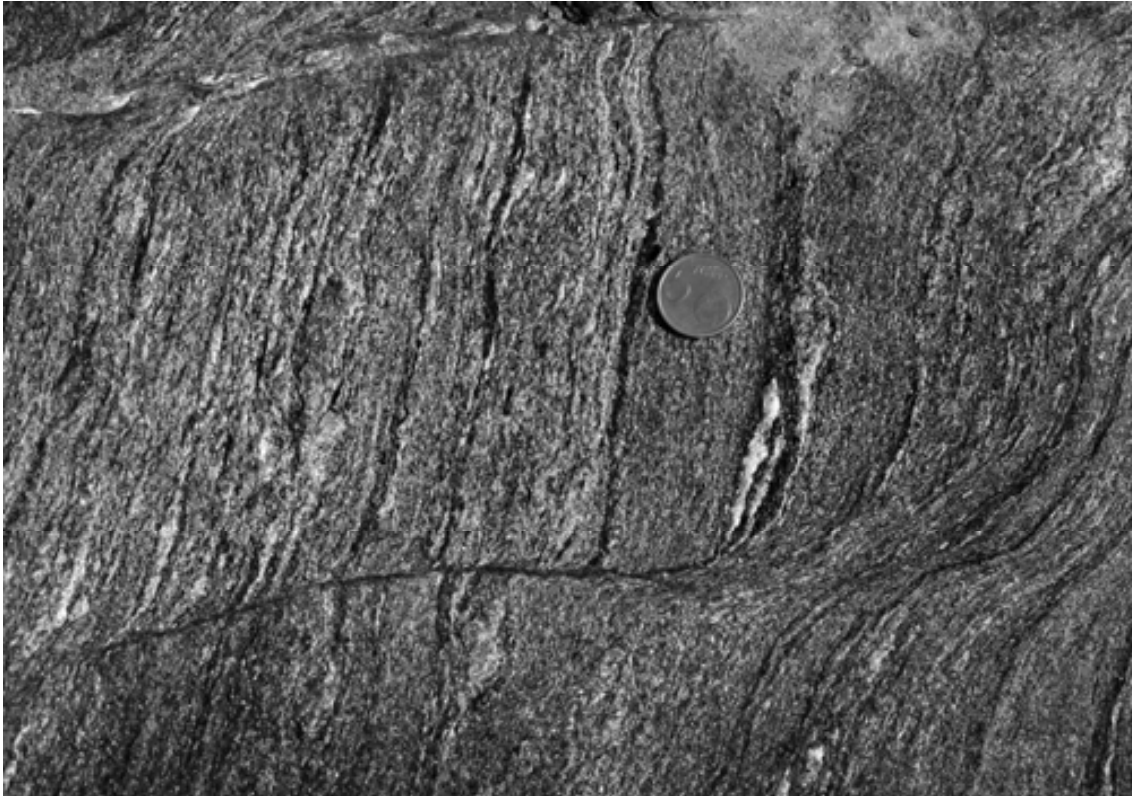
Fig. 3.1. Example of localisation of deformation in amphibolite schists (Cap de Creus, NE Spain). The shear band marked by a tight discontinuity of the medium shows a ductile/plastic front of propagation and bending of anisotropy.
