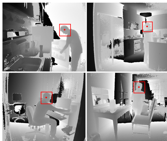
Figure 1: Head detection results (head center and head bounding box depicted as a red dot and rectangle, respectively) on sample depth frames taken from the Watch-n-Patch dataset, that contains kitchen (first row) and office (second row) daily activities acquired by a depth sensor ( i.e. Microsoft Kinect One ).
