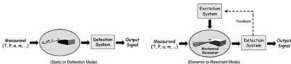
Figure 1.2.1 Schematic representation of the static and dynamic operation modes.
