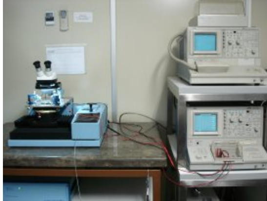
Figure 4.1 Instrumental setup for high-voltage reverse measurements at the power lab.
