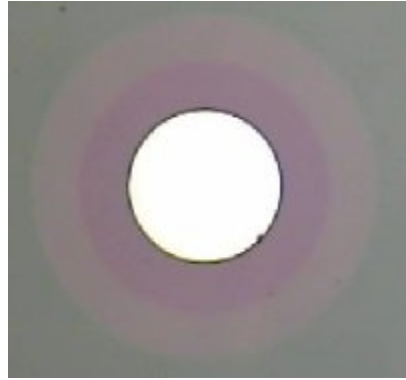
Figure 4.6 Optical image of a fabricated diode with double JTE in embedded configuration ( L_{JTE1}=65\mu\text{m} , L_{JTE2}=125\mu\text{m} ). The two different concentric implanted zones can be clearly distinguished.
