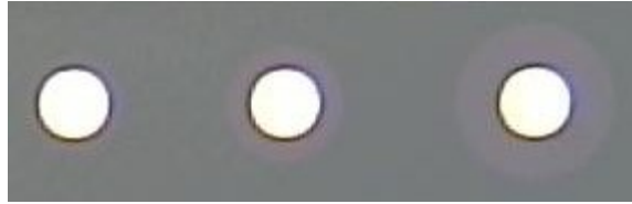
Figure 4.2 Optical photo of the fabricated diodes with different lengths of the JTE
