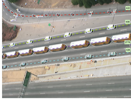
Fig. 1. Different vehicles and its trajectories detected by our approach. From top to bottom: vehicle 422 corresponds to the moto class, the trajectory 408 is a van, a truck can be observed with the vehicle 2776 and the vehicle 426 is a car.
